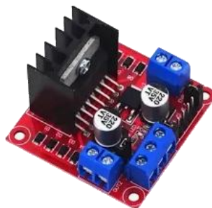
Figura 3: Drive Ponte H
