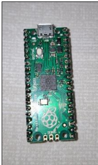
Figura 20 - Raspberry pi pico
