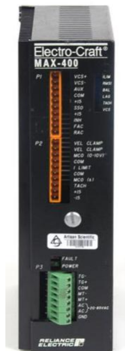
Figura 28 - Servo Drive Reliance Electro-Craft MAX-400
