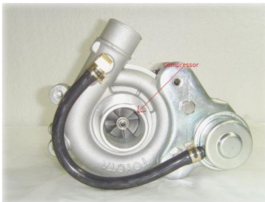
Fig. 28 – Compressor instalado no turbocompressor.
