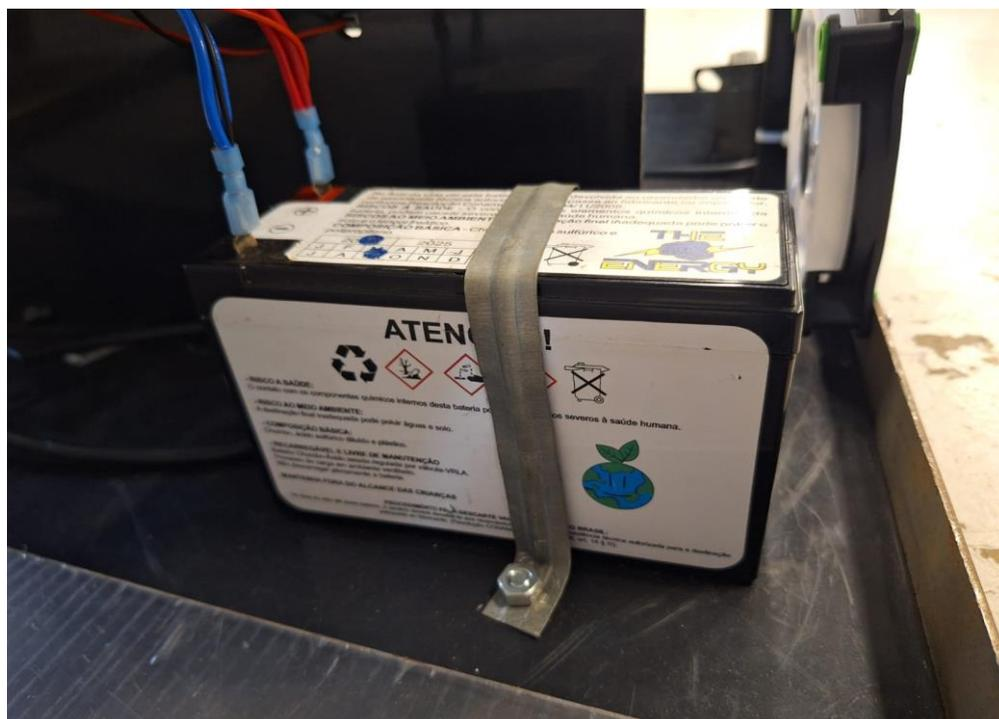
Figura 17 – Bateria Nobreak 12v/7ah
