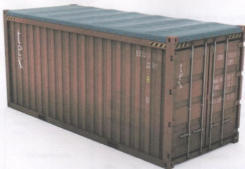
Figura 10: Container Open Top
