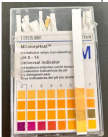
Figura 16. Fita indicando o pH 5,0
