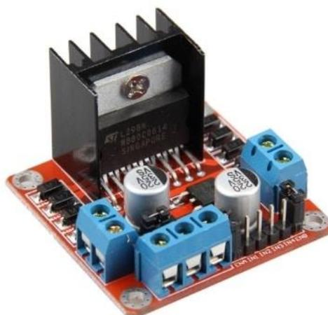
Figura 18: Driver Motor Ponte H – L298N, FONTE: FILIPEFLOP.
