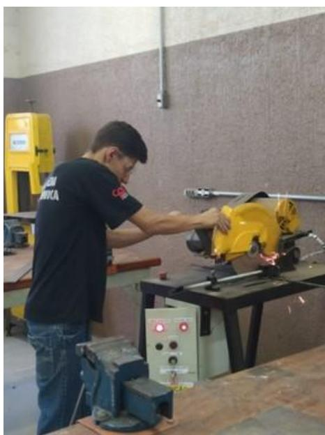
Figura 9: cortando as colunas guias.
