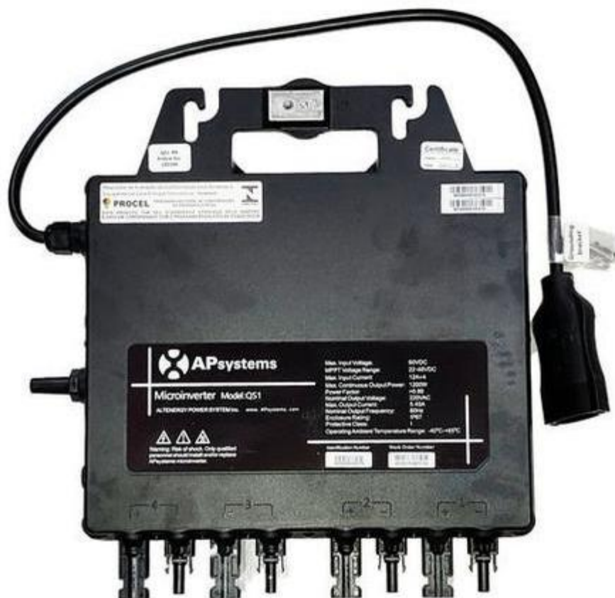
Figura 7.5. Microinversor solar APsystems
