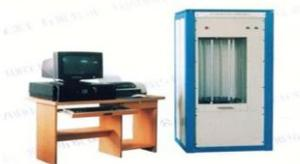
Fully Automatic Filament Crimp Retraction Tester
