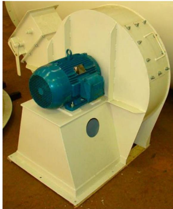
Figura [07]: Motor do exaustor industrial.<sup>[11]</sup>
