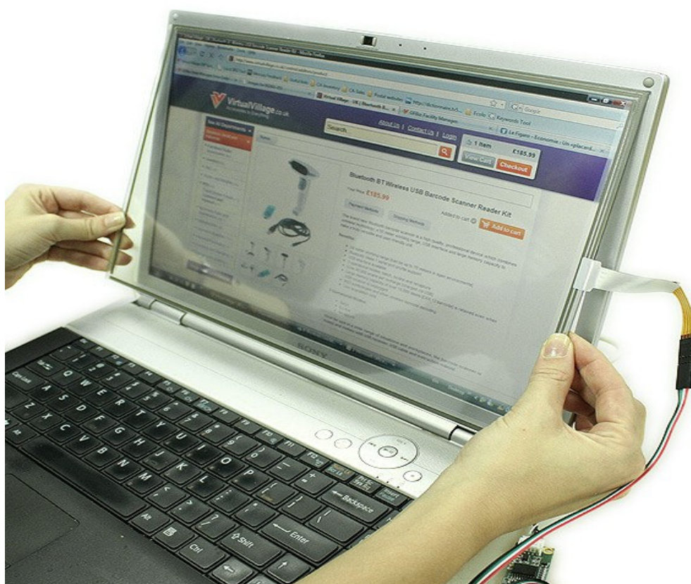
Figura 21: USB Panel kit set sendo instalado, http://www.virtualvillage.com/15-touch-panel-kit-for-interactive-pc-display-007900-006.html
